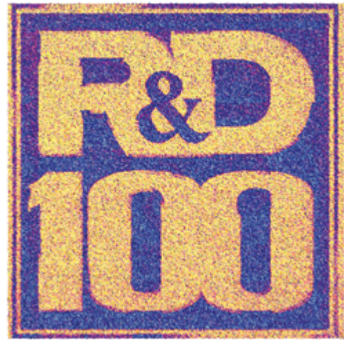
Figure 7: R&D 100 logo written on a sol-gel PZT thin film by PFM lithography. PFM phase is overlaid on top of the rendered topography, 25 \mu\text{m} scan. Oak Ridge and Asylum Research were awarded an R&D100 award for Band Excitation in 2008.
