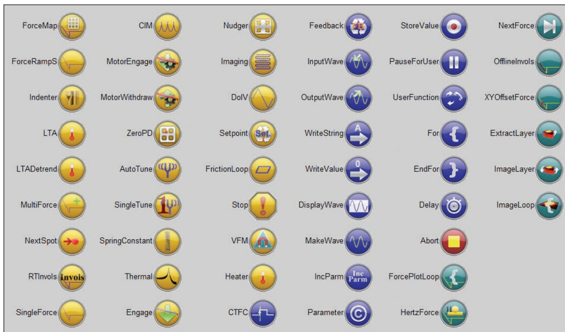
Figure 1: Standard MacroBuilder “Modules” available to users. These Modules can be combined in any number of ways to automate measurements by simply dragging and dropping the Modules into a MacroBuilder Macro sequence. Advanced users can create their own Modules or work with our programmers to develop new Modules.
