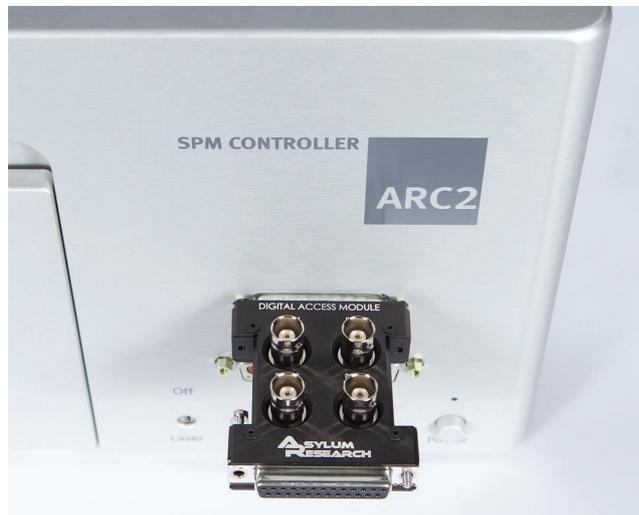
*The Digital Access Module easily plugs into the expansion slot in the front of the ARC2™ Controller.*
